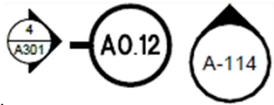
Fig. 2. Three examples of a text and symbol callout referring to another location within a blueprint [1]
