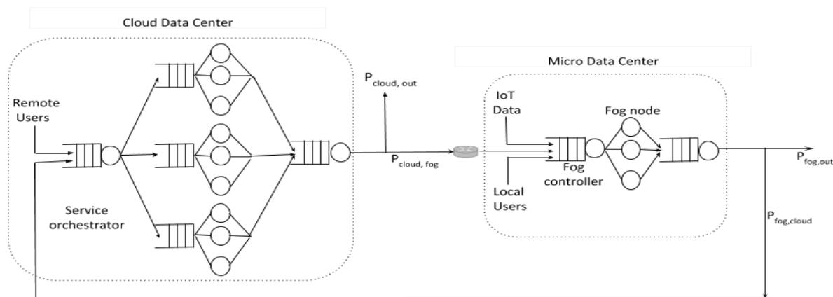
Figure3: Model of IoT Middleware using queuing network
