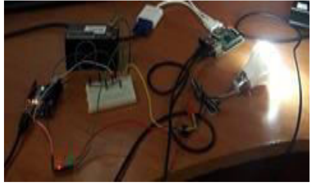
Fig 5. Hardware configuration setup Arduino sense the current and voltage value through Analog pins. With the help of these values, Arduino programing calculates the power and energy. Output is send to the Raspberry through USB cable. Raspberry pi is considered as the server. The monitor displays the web page and cloud data. The components with specification used in proposed system are listed in Table I below
