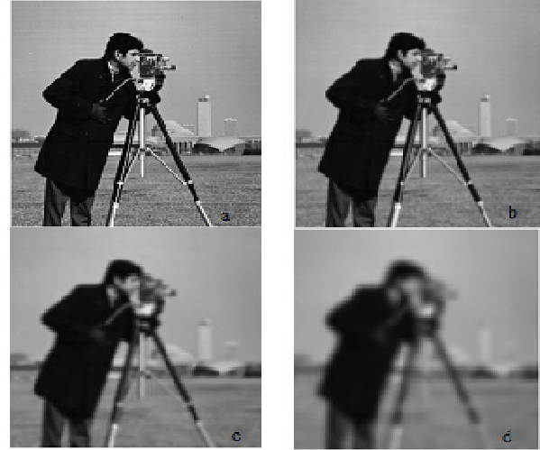
Fig 1: Illustration of Gaussian Scale a. Original Image Filtered Image when b. \sqrt{V} = 1 c. \sqrt{V} = 2 d. \sqrt{V} = 4
