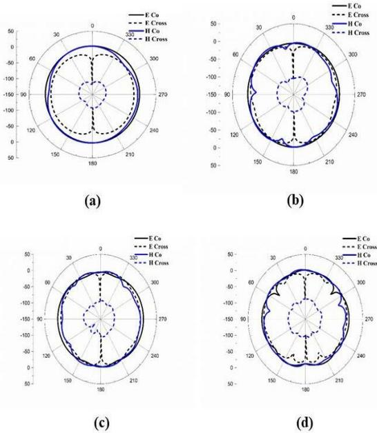
**Fig. 7.** Suggested Antenna Co and cross polarization at 10, 20, 30 and 40 GHz
