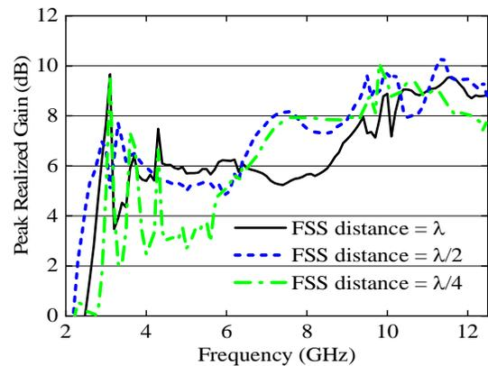
Fig. 11. Realized gain of the suggested antenna at different distance from the FSS
