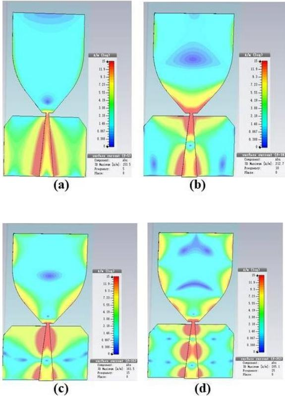
Fig. 4. Suggested Antenna Current distribution
