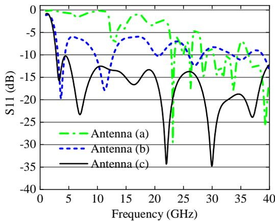
Fig. 2. Suggested Antenna S-parameters
