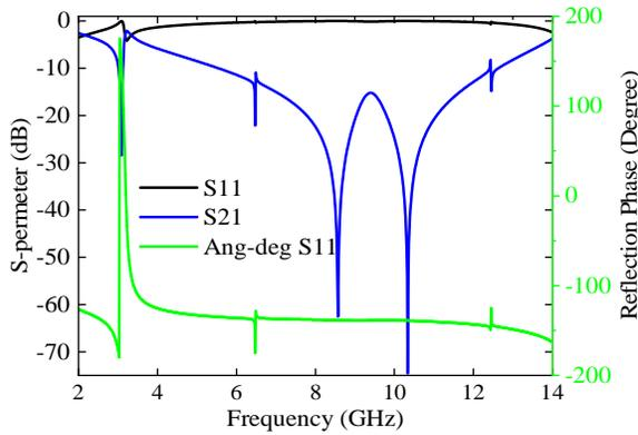
Fig. 10. FSS Transmission and reflection coefficients
