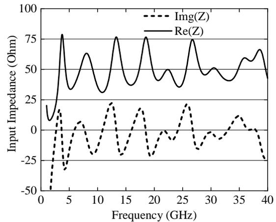
Fig. 6. Suggested Antenna Input Impedance
