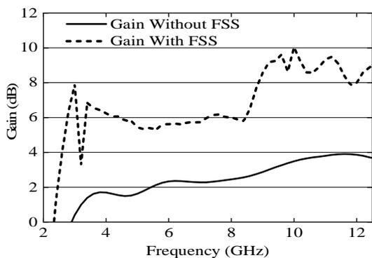
Fig. 12 Suggested antenna Gain with and Without FSS.
