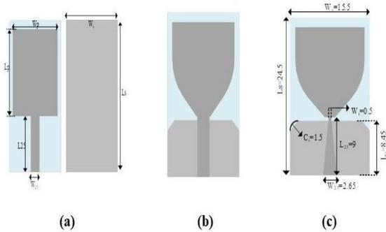
Fig. 1. Suggested Antenna Design Steps (a-c)
