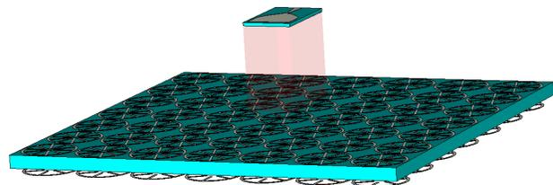
**Fig. 9.** Proposed antenna with FSS
