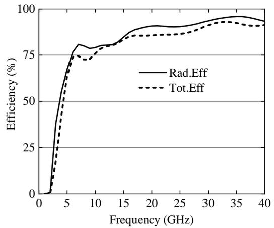
Fig. 5. Suggested Antenna Rad. And Tot. Efficiency
