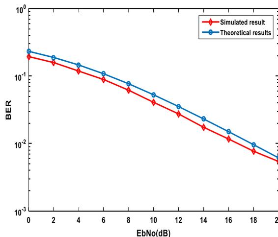
Figure 9 BER against SNR with 16-QAM
