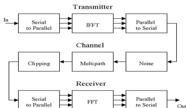
Figure 6 Block diagram of OFDM system [11]
