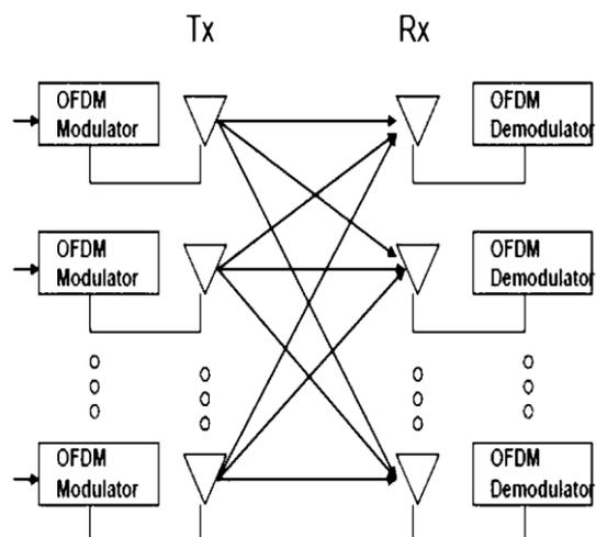
Figure 8 MIMO OFDM structure [9]
