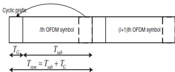
Figure 7 OFDM signal with cyclic prefix [13]
