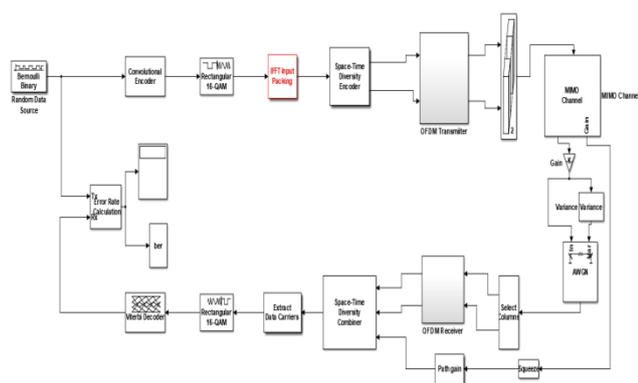
Figure 12 Simulink model of 2x2 MIMO-OFDM system
