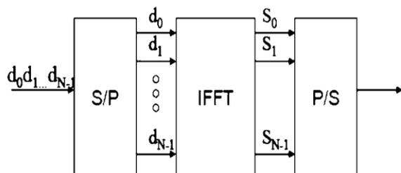
Figure 4 Basic Structure of OFDM transmitter system [9]
