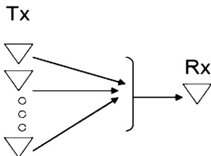
Figure 3 Basic structure of transmit selection diversity
