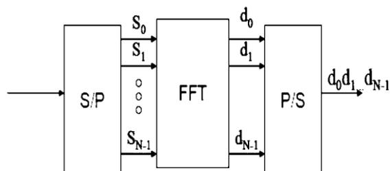
Figure 5 Basic structure of OFDM receiver system [9]
