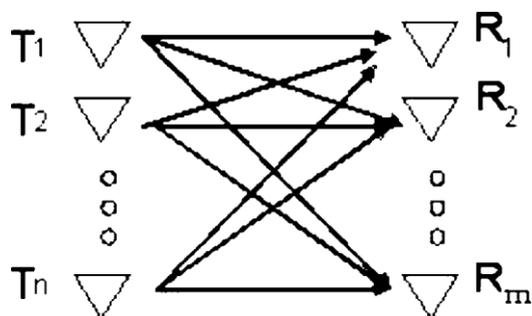
Figure 2 Basic MIMO structure
