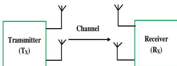
Figure 1 Illustration of MIMO system
