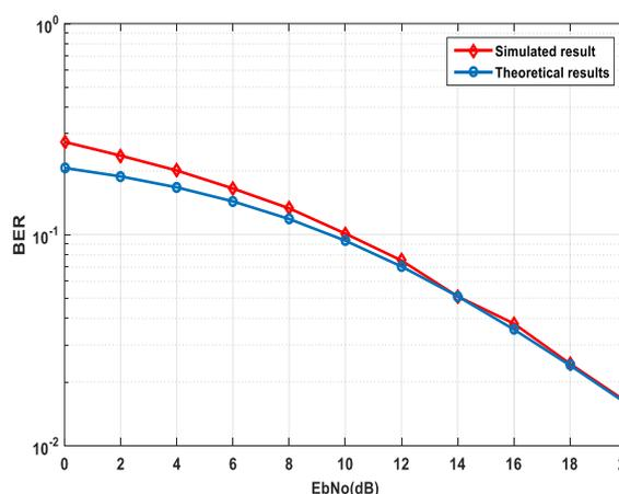
Figure 11 BER against SNR with 128-QAM
