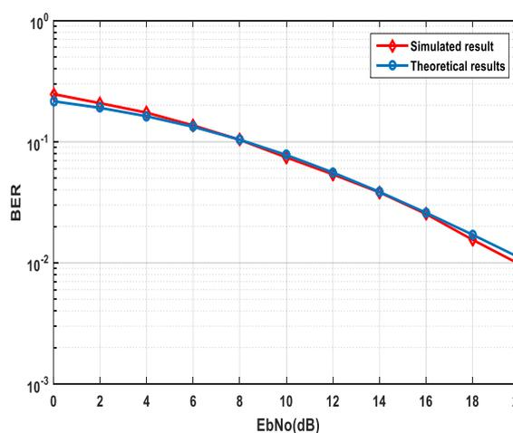
Figure 10 BER against SNR with 64-QAM
