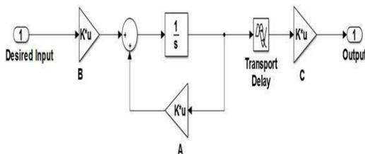
Fig. 2 System state-space model in Simulink
