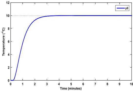
Fig. 8 Temperature response (open loop)
