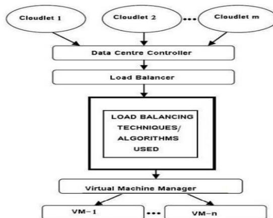
**Fig-2 (Load Balancing Algorithm execution)**
