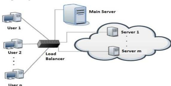
**Fig-1 (Load Balancing in Cloud Computing environment)**
