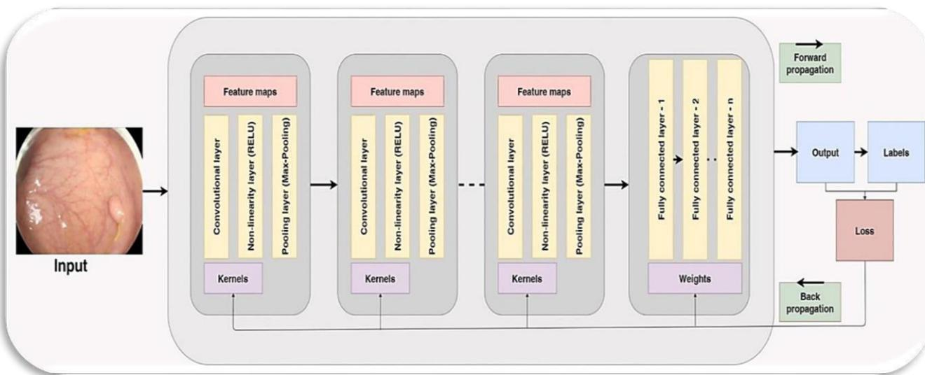
**Fig.2 Convolutional Neural Network Architecture [6]**
