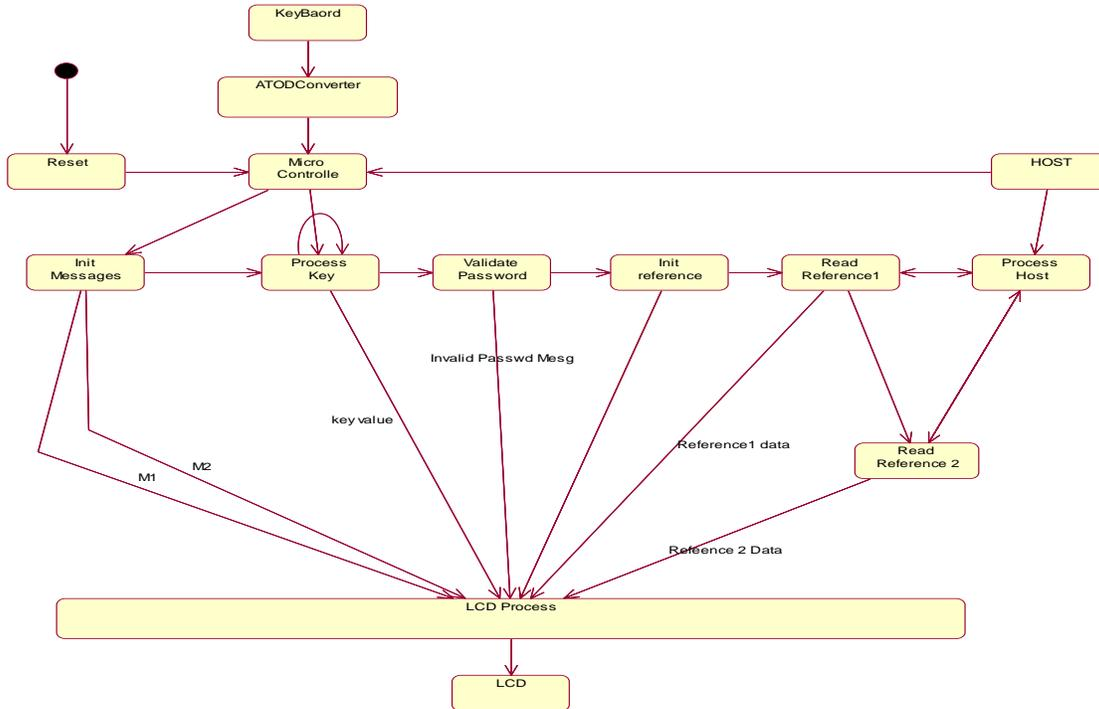
Figure 4.12 Sub-Level State diagrams for the Top Level State Initialization and Main Control
