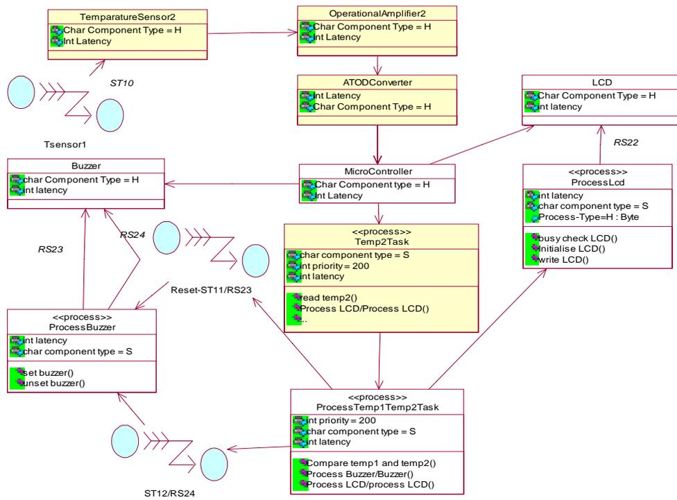
Fig 4.4 Class Diagram for processing Temperature Thresholds
