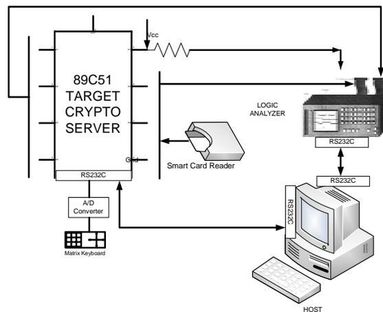
**Figure 5.1 Experimental setup for attacking through power analysis**
