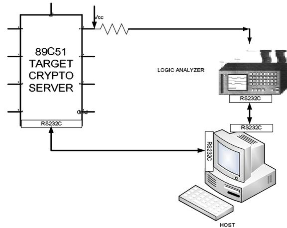
Figuer.4.1 experimental setup of power analysis attacks
