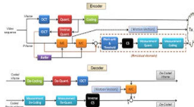
Fig.3. Sparse sampling in video encoding
