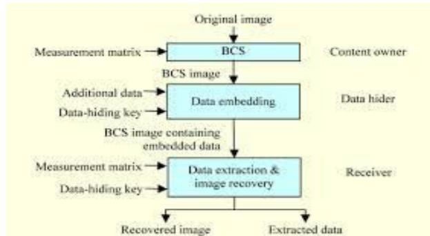
Fig.5. Sparse sampling in image encryption
