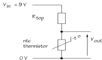
Fig. 4. Circuit diagram of NTC Thermistor
