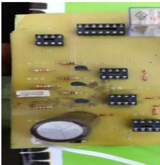
Fig 6. Fixing the components on the PCB
