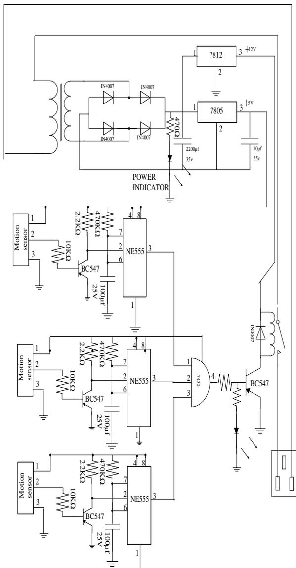
Fig 1. Control Unit Circuit diagram
