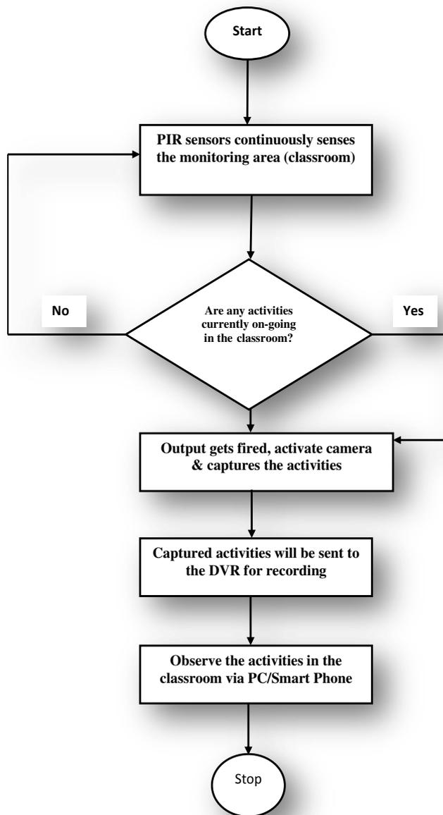
Fig 2. Flowchart for Proposed System Working Mechanism
