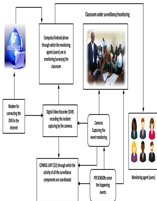
Fig 4. Proposed Systems Architecture & Data Flow
