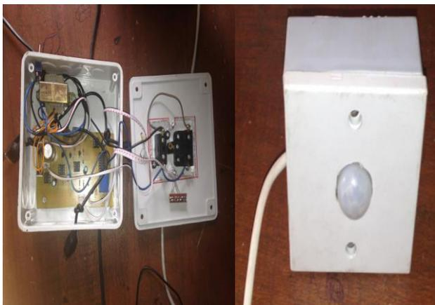
Fig 8: Control system and PIR Sensor
