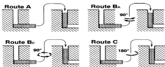
Fig:1 The four fundamental processing routes in ECAP
