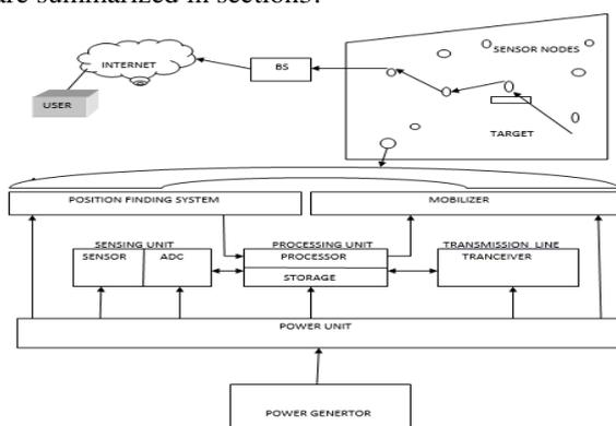
Fig 2. Components of Sensor Nodes
