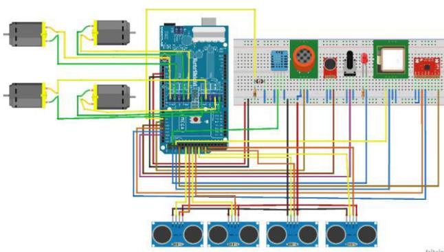
Figure 5. Arduino IoT II device scheme.
