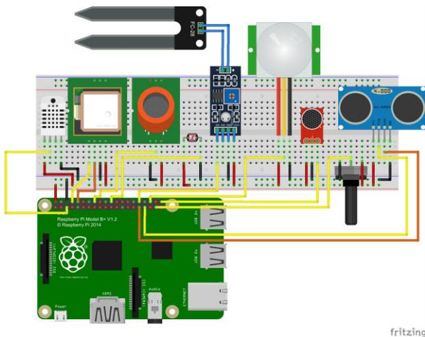
Figure 3. Raspberry IoT I device scheme.
