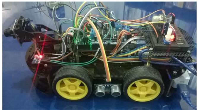
Figure 6. Construction of IoT II device with Arduino.
