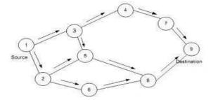
Fig 3: The Route Request packets flooding in AODV
