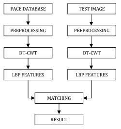
Fig.1. Block diagram of HDFRS
