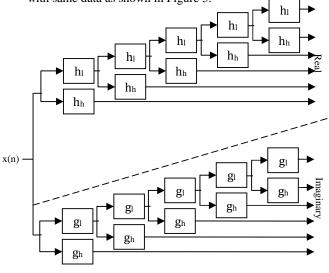
Fig.5. Filter Bank of DT-CWT
