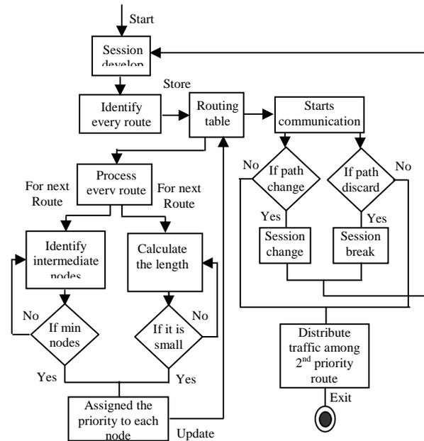
Figure 2. Flow Chart of proposed algorithm
