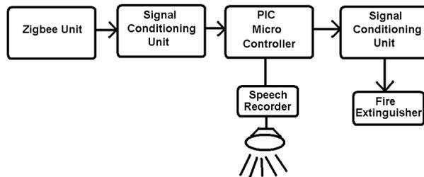
Figure 4 Extinguishing Node
