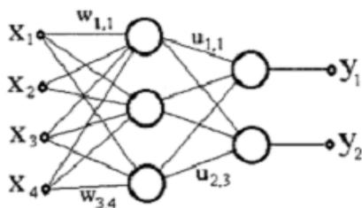
Fig 2.2: A two layer feed forward neural network
