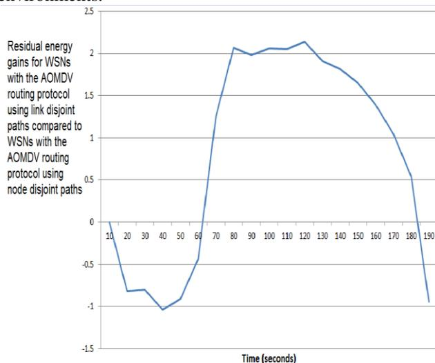
Fig. 27 Differences in Residual Energy of a WSN using the AOMDV Routing Protocol along Link Disjoint Paths and a WSN with the AOMDV Routing Protocol along Node Disjoint Paths
