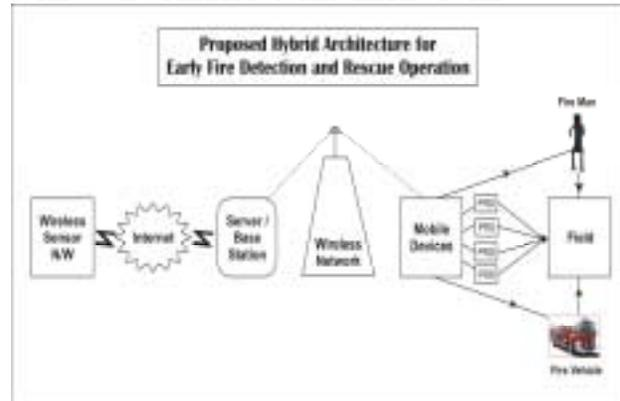
Fig 4 Hybrid architecture of Early Fire Detection.
