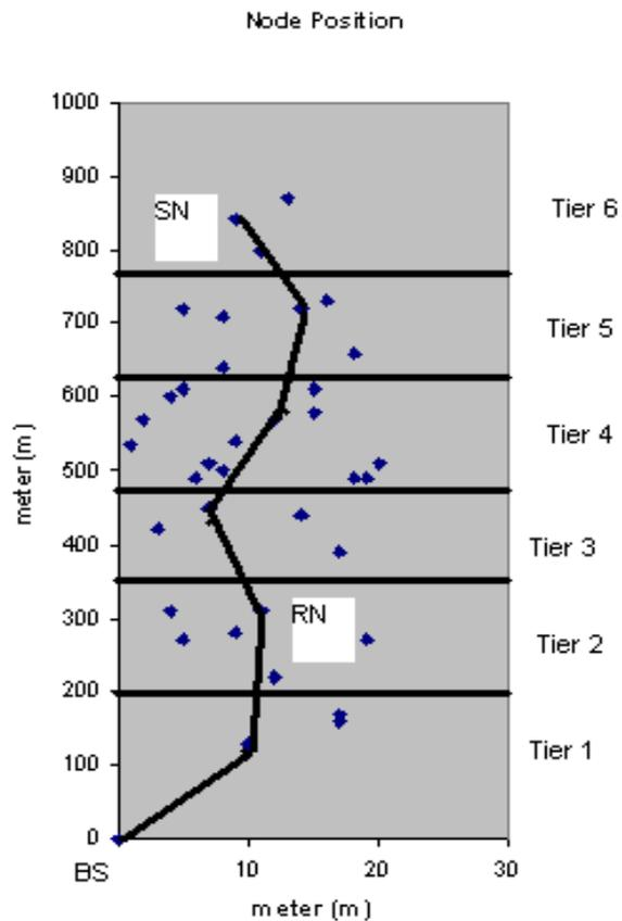
Fig. 1 Nodes and tierNum as distance to BS (SN = Sensing Node, RN = Routing Node and BS = Base Station).
