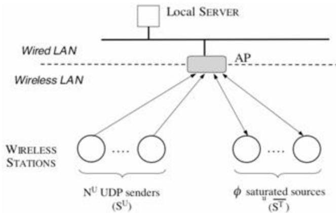
Fig. 2. The equivalent network model: network and traffic configurations
