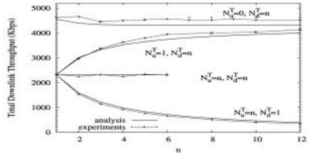
Fig. 3. Comparison of model predictions and measured total downlink throughput.
