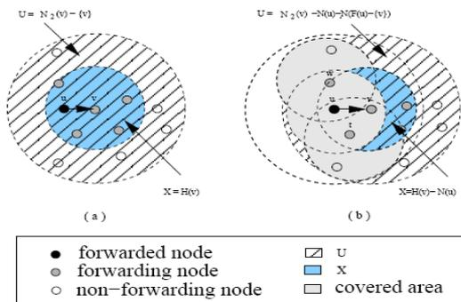
Fig 4: Illustrations of the forwarding node set selection process of the EDCB algorithms.
