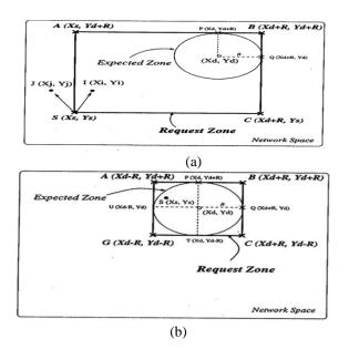
Figure 1.6(a): Source node outside the expected zone Figure 1.6(b): Source node within the expected zone
